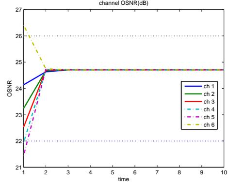
Fig. 3. OSNR equalization: Original
