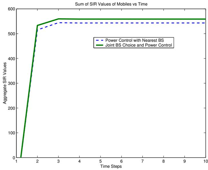
**Figure 16:** Sums of the SIR values of mobiles (in dB) with respect to time for power control with nearest BS choice and hybrid power control scheme.
