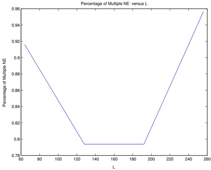
**Figure 6:** Percentage of mobile locations with multiple NE solutions for different values of L.
