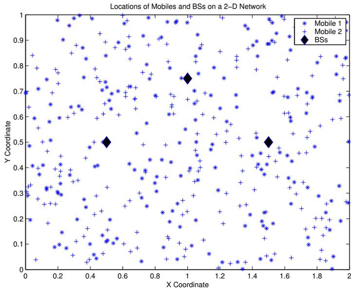
**Figure 12:** Randomly generated locations of two mobiles on a 2-D wireless network with 3 BSs.
