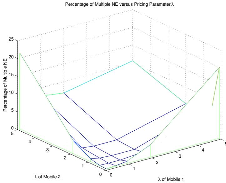
**Figure 10:** Percentage of mobile locations with multiple NE solutions for different values of  $\lambda_1$  and  $\lambda_2$  on a 2-D wireless network.
