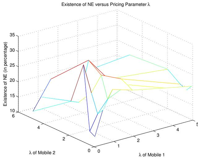
**Figure 11:** Percentage of mobile locations with NE solutions in the case of quadratic pricing function,  $P_i = \lambda_i p_i^2$ , for different values of  $\lambda_1$  and  $\lambda_2$  on a 2-D wireless network.
