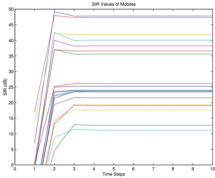
**Figure 15:** SIR values of mobiles (in dB) with respect to time.
