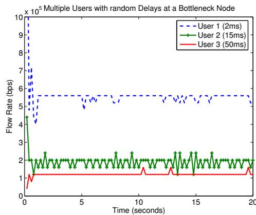
Fig. 3. Three out of 20 flows with various propagation delays ( $2ms$ ,  $15ms$ , and  $50ms$ ) sharing a  $5Mbps$  bottleneck link.
