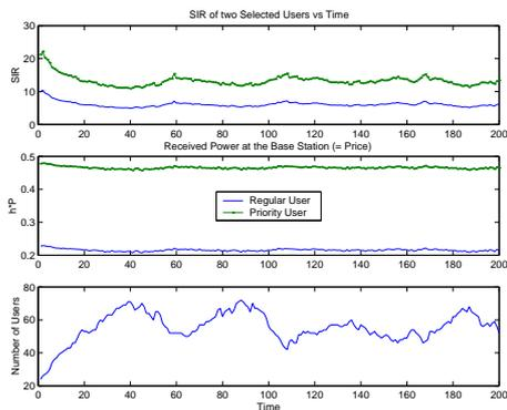
**Figure 3:** SIR and power levels at the base station of a priority and a regular user versus time.
