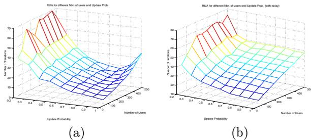
**Figure 2:** Convergence rate for different  $\pi_i$ 's and  $M$ 's in (a) delay-free (b) delayed cases.
