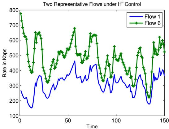
Fig. 6. The rates of representative flows 1 and 6 on network 1 under  $H^\infty$ -optimal control.
