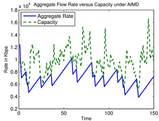
Fig. 9. The aggregate flow rate and the available capacity on network 1 under AIMD control.
