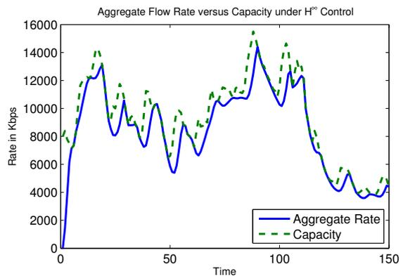
Fig. 5. The aggregate flow rate and the available capacity on network 3 under  $H^\infty$ -optimal control.
