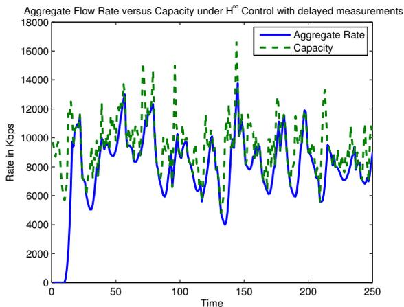
Fig. 17. The aggregate flow rate and the available capacity on network 1 under  $H^\infty$ -optimal control and randomly delayed measurements.
