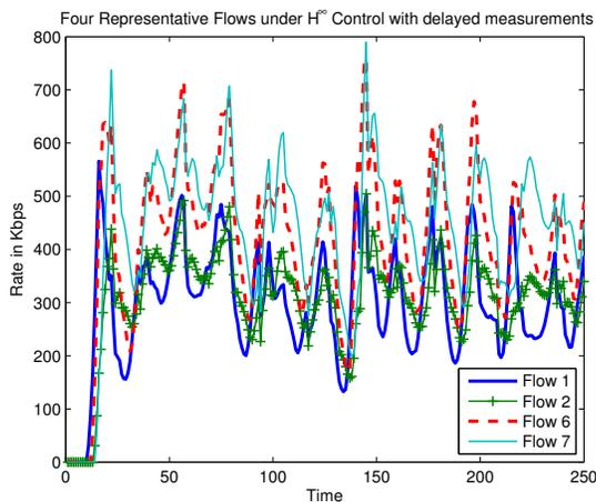
Fig. 16. The flow rates of individual flows on network 1 under  $H^\infty$ -optimal control. In accordance with Table 1, flows 1, 2, 6, 7 experience individual measurement delays of 2.5, 10, 7.5, 12.5 ms, respectively.
