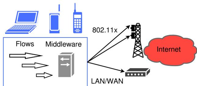
Fig. 1. The envisioned middleware architecture utilizing a lightweight tool to estimate the bandwidth and delay of the heterogeneous networks accessible by the mobile device.
