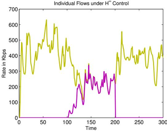
Fig. 12. The flow rates on network 1 under  $H^\infty$ -optimal control and varying number of active devices.
