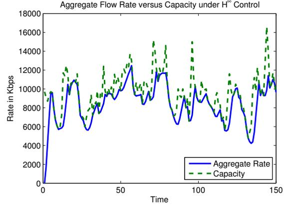
Fig. 3. The aggregate flow rate and the available capacity on network 1 under  $H^\infty$ -optimal control.
