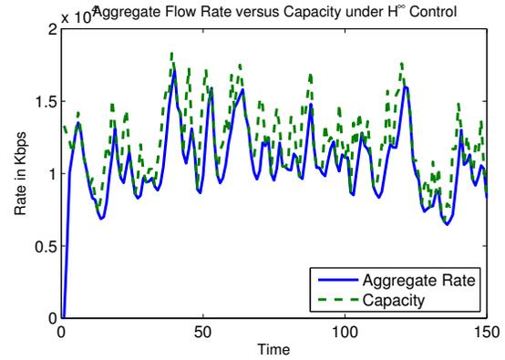
Fig. 4. The aggregate flow rate and the available capacity on network 2 under  $H^\infty$ -optimal control.
