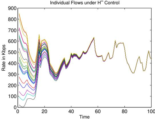
Fig. 11. The rates of individual flows with random starting points on network 1 under  $H^\infty$ -optimal control.
