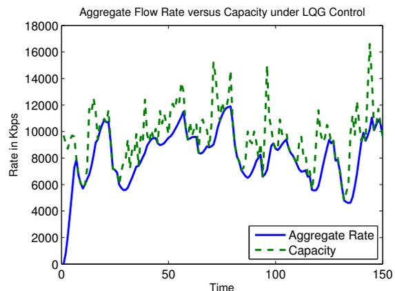
Fig. 10. The aggregate flow rate and the available capacity on network 1 under LQG control.
