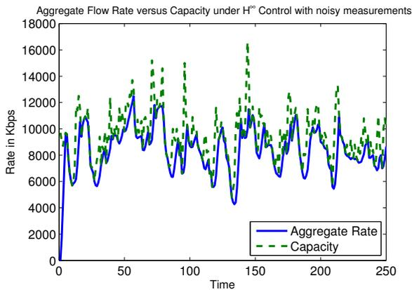
Fig. 15. The aggregate flow rate and the available capacity on network 1 under  $H^\infty$ -optimal control and Gaussian measurement noise  $\mathcal{N}(0, 200^2)$ .
