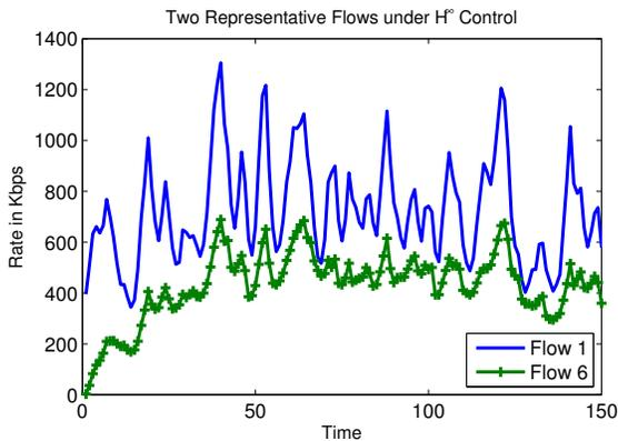
Fig. 7. The rates of representative flows 1 and 6 on network 2 under  $H^\infty$ -optimal control.
