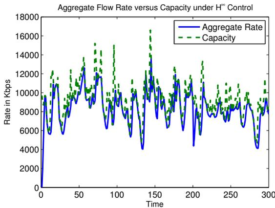
Fig. 13. The aggregate flow rate and the available capacity on network 1 under  $H^\infty$ -optimal control and varying number of active devices.
