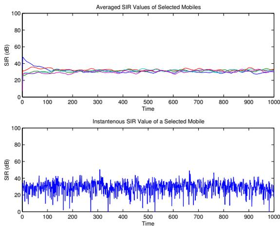
Fig. 9. SIR and averaged SIR values of selected mobiles (in dB) with respect to time under imperfect feedback information.
