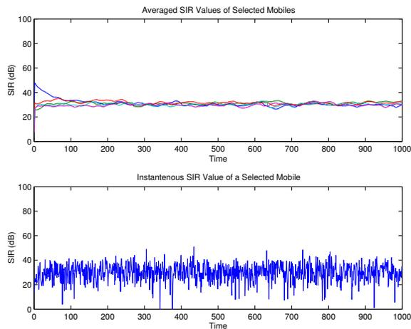
Fig. 4. SIR and averaged SIR values of selected mobiles (in dB) with respect to time.
