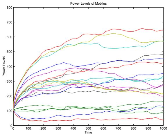
Fig. 8. Power levels of selected mobiles with respect to time under imperfect feedback information.
