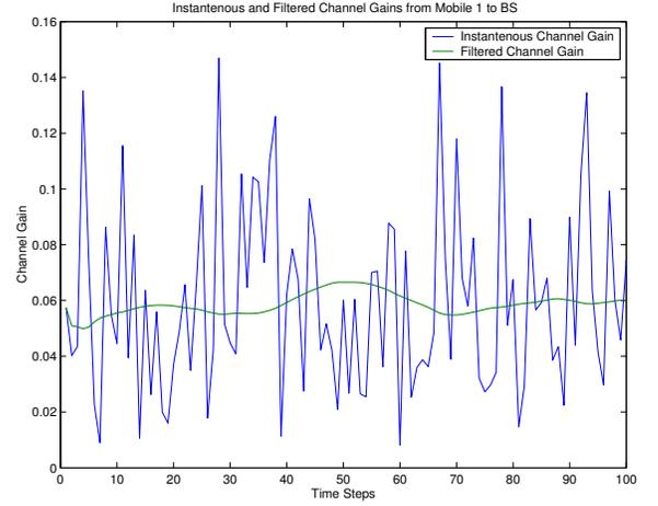
Fig. 2. Instantaneous and filtered channel gain from mobile one to its respective BS.
