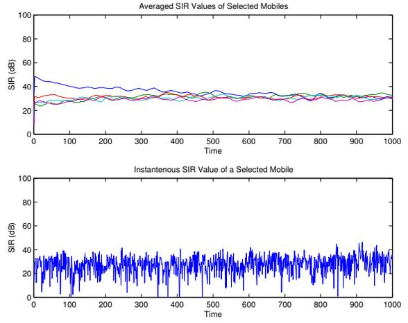
Fig. 7. SIR and averaged SIR values of selected mobiles (in dB) with respect to time.
