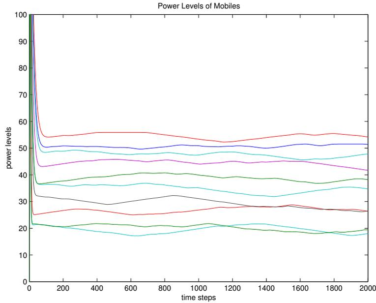
Fig. 5. Power levels of 10 selected mobiles with respect to time.
