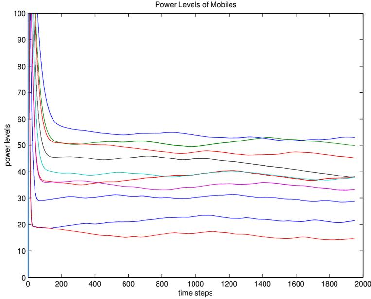
Fig. 7. Power levels of 10 selected mobiles with respect to time under a communication delay of 50 steps.
