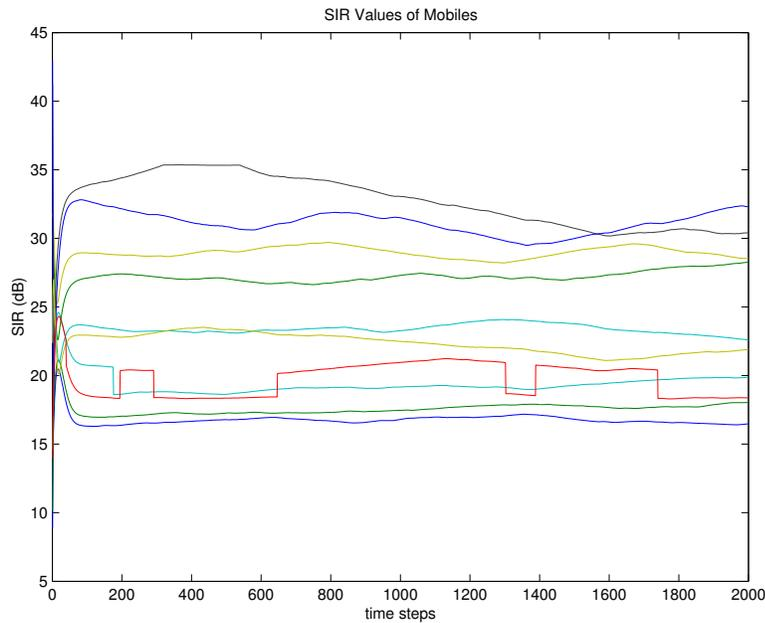
Fig. 6. SIR values of 10 selected mobiles (in dB) with respect to time.
