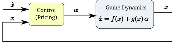
Fig. 2. Feedback control of the game (NE,  $\mathbf{x}^*$ ) using pricing  $\alpha$  as the control parameter and  $\hat{\mathbf{x}}$  as the desired reference signal.
